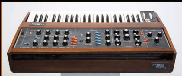
Pictured above and below: The Minimoog's control panel features knobs to adjust volume and resonance, and can be left upright or folded back.
